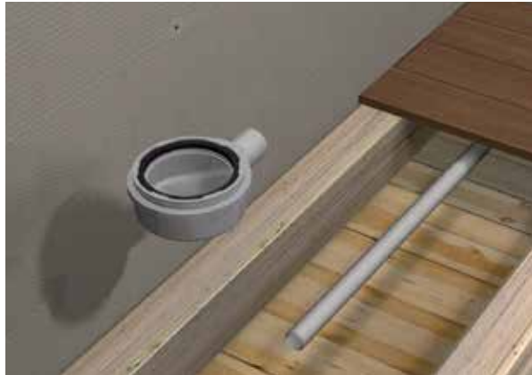
2. Install the waste ensuring adequate run off.
