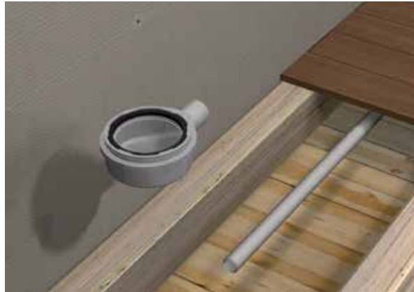
2. Install the waste ensuring adequate run off.
