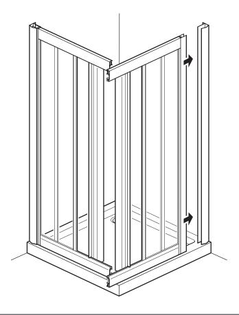
Insert the sides into the wall channels and roughly position on the tray.
