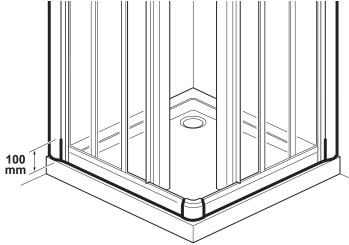
Before sealing you must make sure that the doors open and close correctly.
