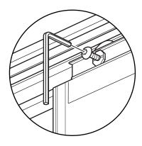
If the doors are not square with the fixed panels or they don't close correctly, one or both of the top sliders should be adjusted.
