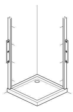
Remove both wall channels from each side of the enclosure. Place each wall channel in position on the tray (10 - 15mm in from the outer edges of the tray), use a spirit level to ensure they are vertical and mark all 8 fixing holes onto the walls (holes inside).
