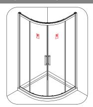
• The "up" arrow on the sliding door should be above, and be on the outside of the enclosure.
