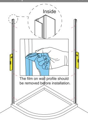
Remove both wall channels from the glass panel frame. **Note:** *Ensure the longer leg of each wall channel is on the inside of the enclosure when fixing.* Place each wall channel in position on the tray (10 - 15mm in from the outer edge of the tray), use a spirit level to ensure that they are vertical and mark all 8 fixing holes onto the wall.
