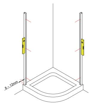
Remove both wall channels from the glass panel frames. Place each wall channel in position on the tray (8 - 12mm in from the outer edge of the tray), use a spirit level to ensure that they are vertical and mark all 6 fixing holes onto the wall.
