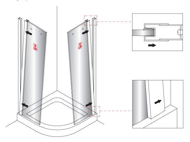
Fix the track to the glass panel with the connectors (F, G) by the allen key (T).
